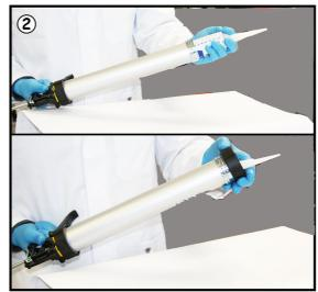
2. Load sausage pack in gun. Screw front cap onto barrel
