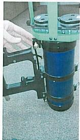
Carefully rotate the forward/reverse switch, clamps/combo trigger and back cap of cylinder in small, incremental steps as the air hose between the switch and back cap are still connected
