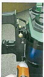
Loosen 4 Allen screws on clamps holding combo trigger to cylinder (do not loosen completely, just enough so the clamps slide freely on the cylinder)
