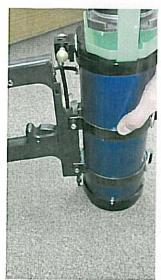
Slide the clamps and combo trigger together towards the back of the gun
